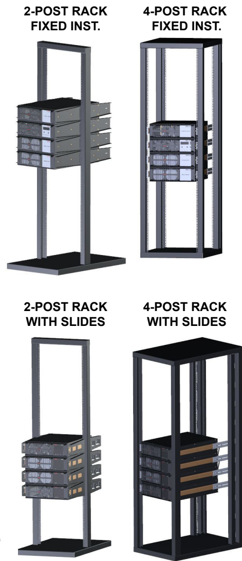
FIGURE 6-6: RACK INSTALLATION OPTIONS
