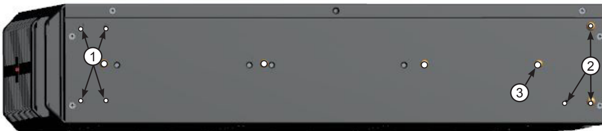
FIGURE. 6-8: RACKMOUNT BRACKET MOUNTING HOLES
