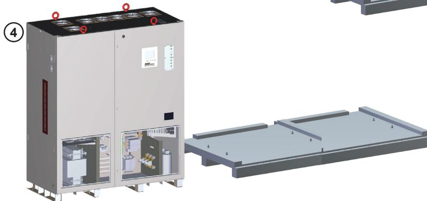
5. Use a forklift or crane to transport the UPS to its installation location. See **Section 8**.
