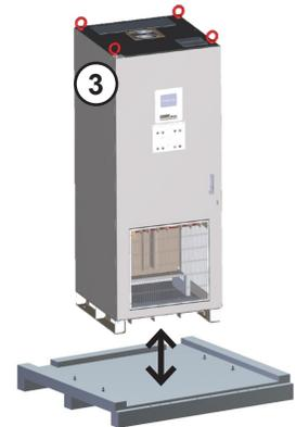
5. Use a forklift or crane to transport the UPS to its installation location. See **Section 8**.
