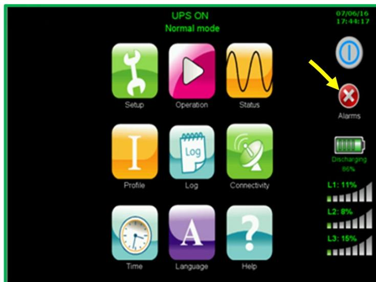
Figure 30: The "alarms" icon indicates alarm conditions
