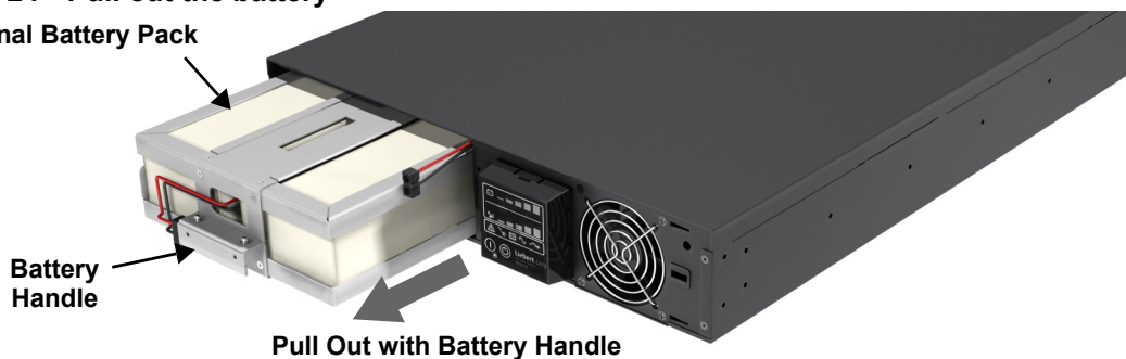
Figure 24 Pull out the battery
