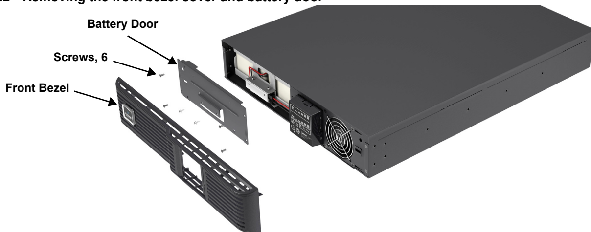
Figure 22 Removing the front bezel cover and battery door
