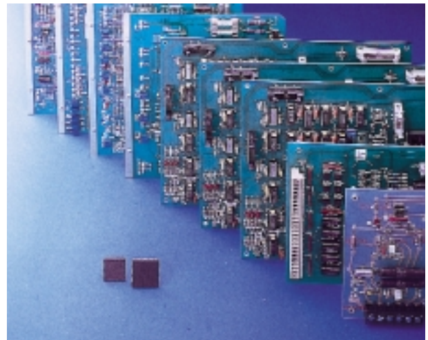
Application-Specific Integrated Circuits (ASICs) reduce the parts count and significantly increase system reliability.
