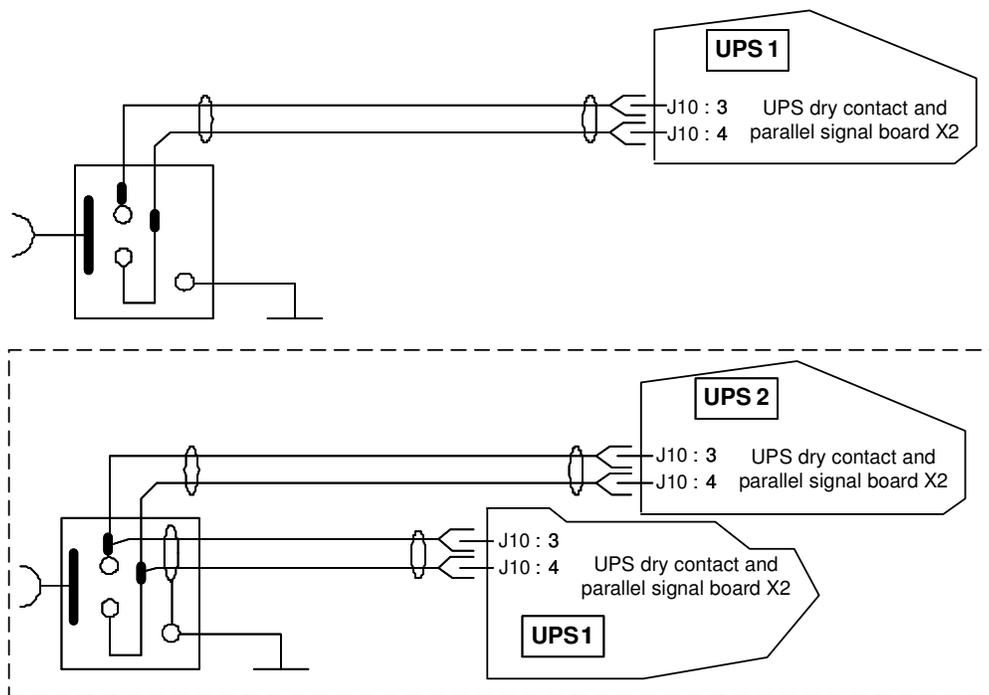
Fig. 3-1: Circuit ram of emergency power off
