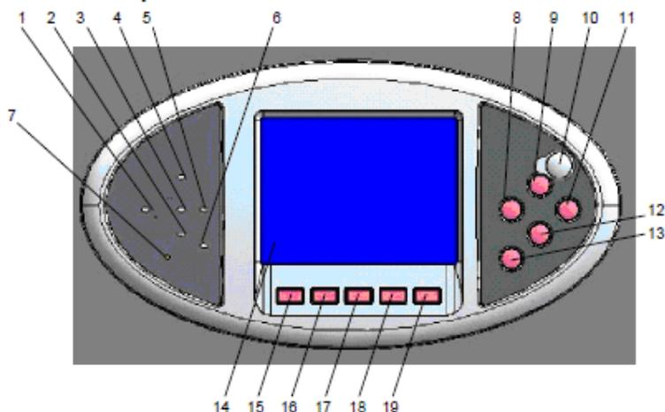
Fig. 7-1: UPS operator control and display panel
