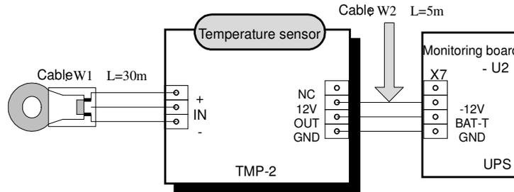
Cable W2 is delivered together with the temperature sensor
