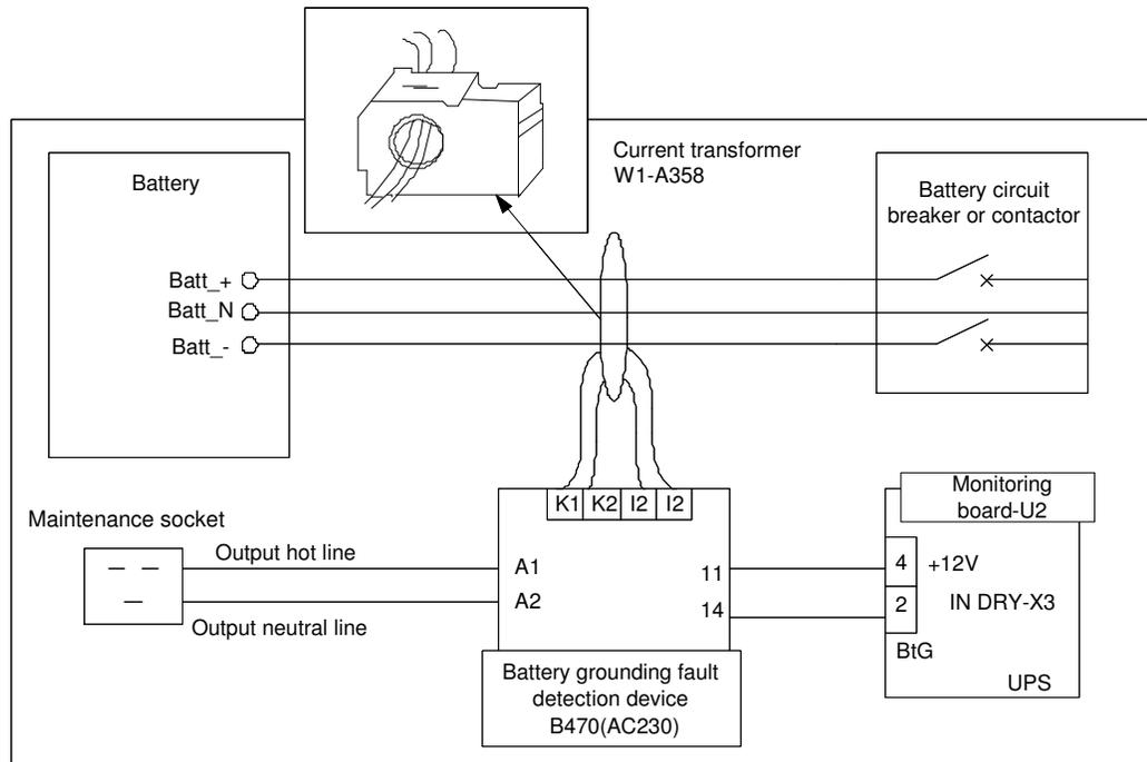
Fig. 8-1: Wiring of battery ground fault detection set
