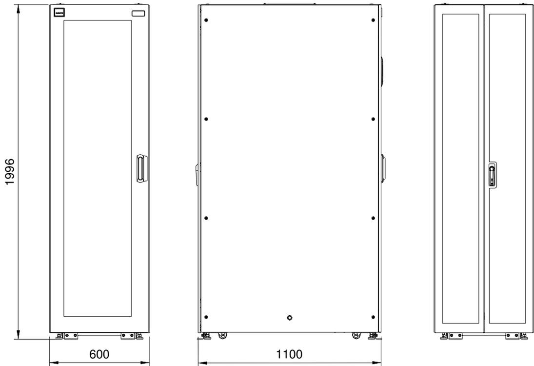
Fig. 4-6: Battery Cabinet External dimensions
