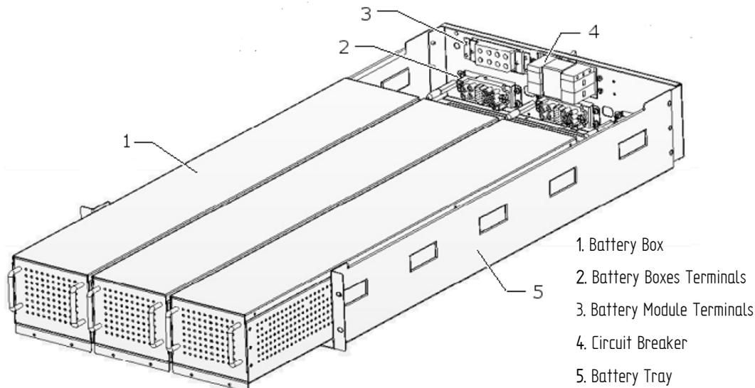
Fig. 4-14: Battery Module
