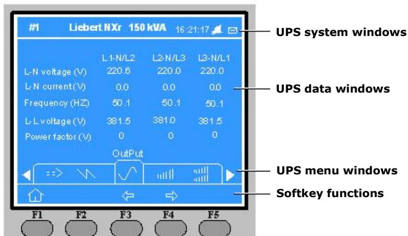
Fig. 7-2: Sections of the LCD and menu buttons
