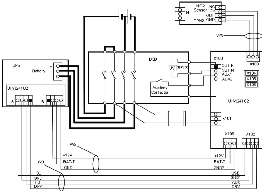
Fig. 4-2: External Battery Connections
