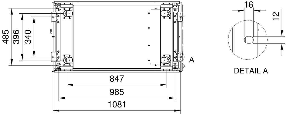
Fig. 4-7: UPS and BC bottom view show the position of casters and fixing holes
