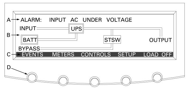
Figure 7-3. Parts of the LCD
