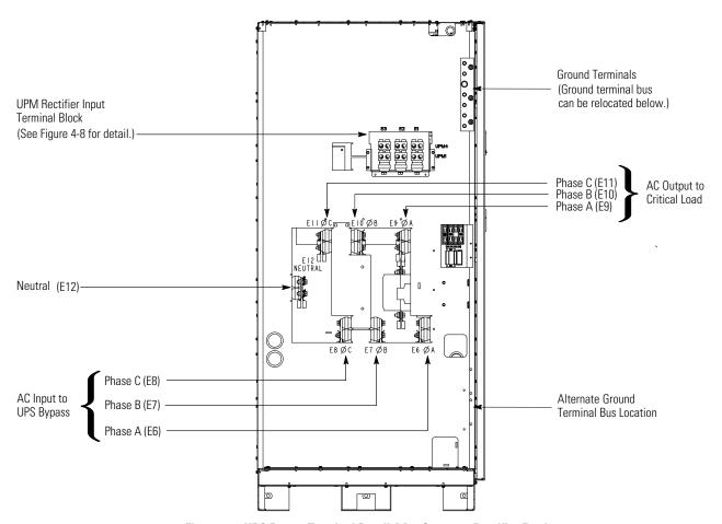
Figure 4-7. UPS Power Terminal Detail AA – Separate Rectifier Feed
