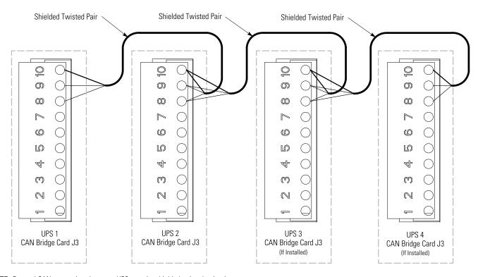
NOTE External CAN connections between UPSs require shielded twisted-pair wire.
