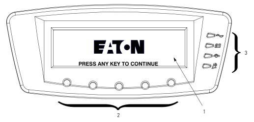
Figure 7-2. UPS Control Panel
