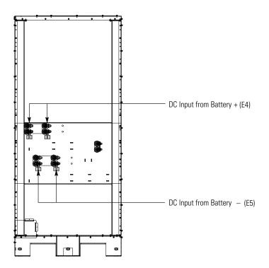
Figure 4-9. UPS Power Terminal Detail BB – Common Battery
