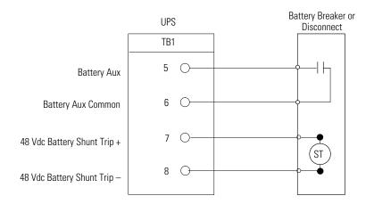
**NOTE** Battery Aux and DC Shunt Trip wiring should be a minimum of 18 AWG.
