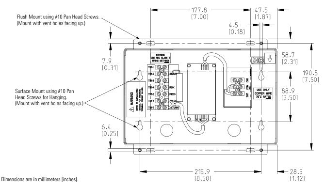
Figure 5-12. Remote Monitor Panel II Dimensions
