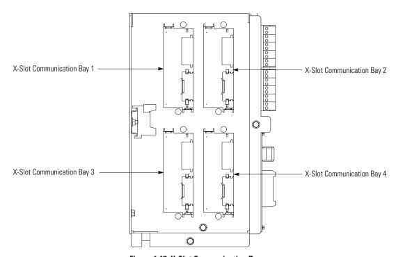
Figure 4-17. X-Slot Communication Bays
