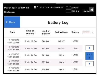
Figure 7-28. Battery Log Detail
