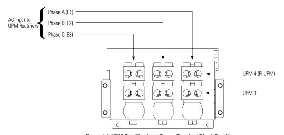
Figure 4-8. UPM Rectifier Input Power Terminal Block Detail
