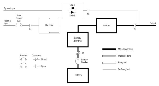
Figure 6-4. Path of Current Through the UPS in Battery Mode
