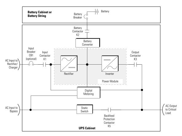
Figure 6-1. Main Elements of the UPS System
