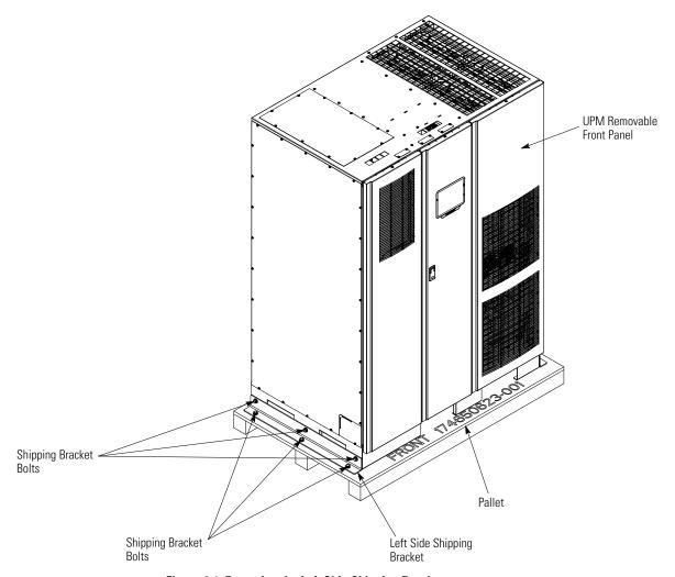
Figure 4-1. Removing the Left Side Shipping Bracket
