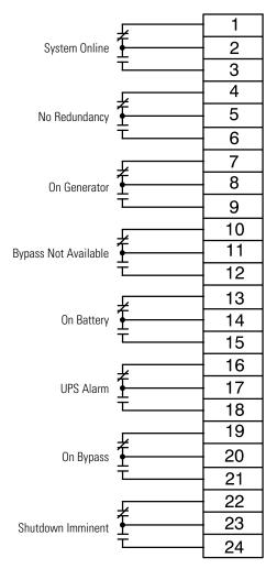
Figure 5-11. Supervisory Contact Module II TB2
