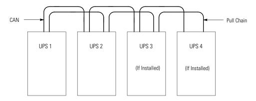
**NOTE** This drawing is for distributed bypass wiring purposes and is not a floor layout plan. UPSs can be placed in any physical order.
