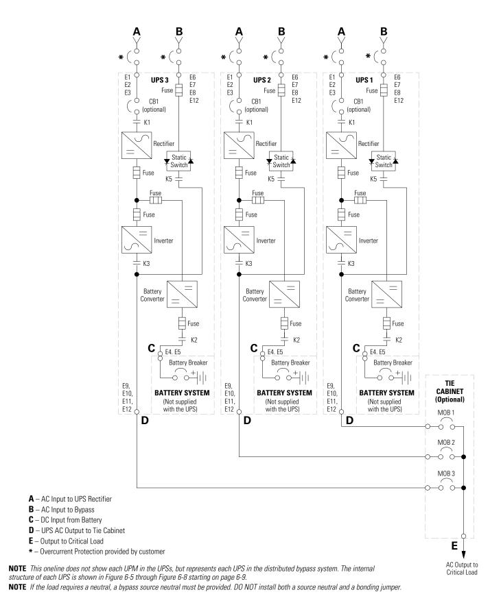
Figure 6-14. Typical Distributed Bypass System (2+1 and 3+0 Configurations)
