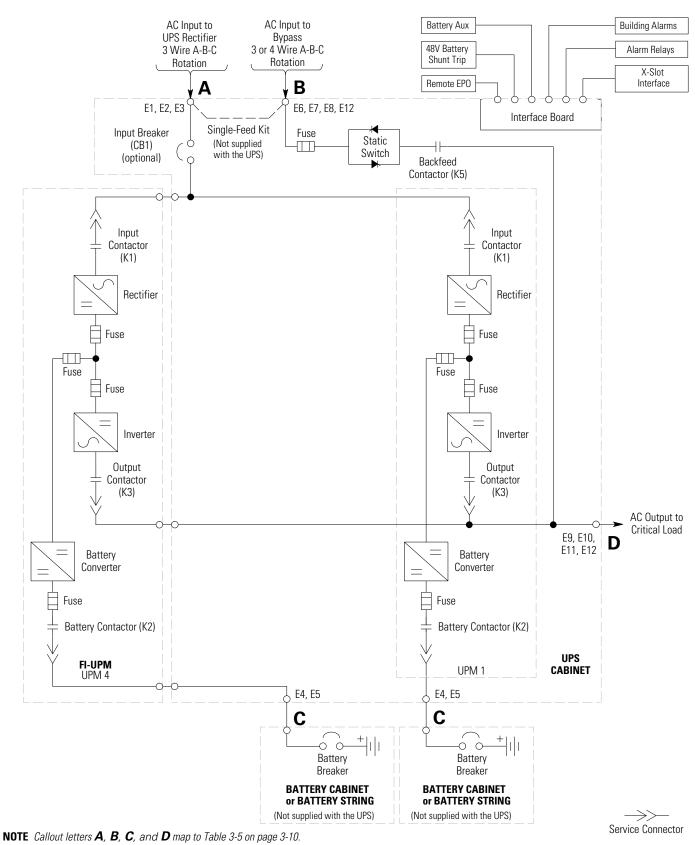
NOTE If the load requires a neutral, a bypass source neutral must be provided. DO NOT install both a source neutral and a bonding jumper.
