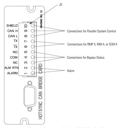
Figure 5-2. Powerware Hot Sync CAN Bridge Card Connections
