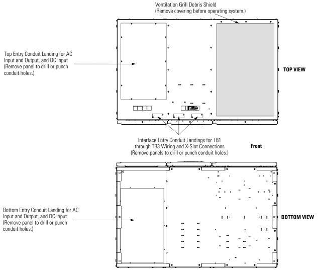
Figure 4-4. Conduit and Wire Entry Locations
