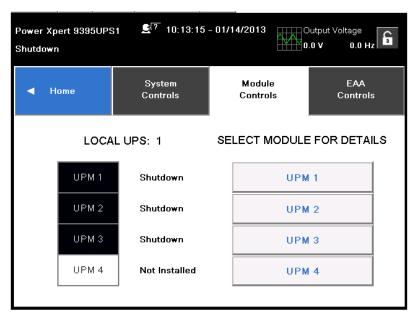
Figure 7-34. Module Controls Screen
