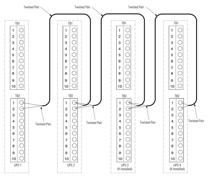
**NOTE** Use twisted-pair wiring between the UPS and MOB AUX contacts.
