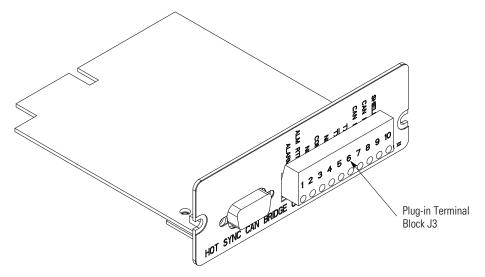
Figure 5-1. Powerware Hot Sync CAN Bridge Card
