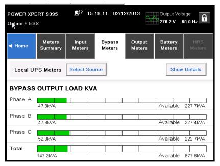
Figure 7-22. Bypass Meters Screen
