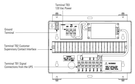
Figure 5-10. Supervisory Contact Module II Terminal Location
