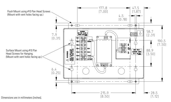
Figure 5-13. Relay Interface Module II Dimensions
