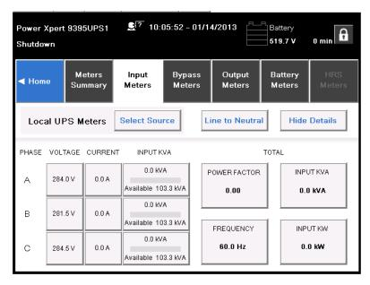
Figure 7-24. Input Meters Detail Screen
