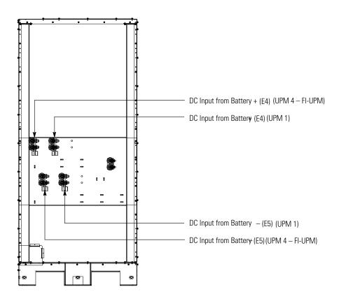
Figure 4-10. UPS Power Terminal Detail BB – Separate Battery
