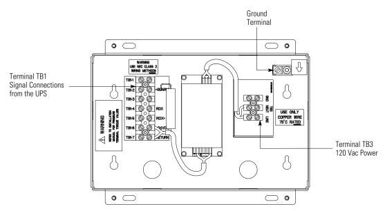
Figure 5-7. Remote Monitor Panel II and Remote Monitor Panel II Terminal Locations
