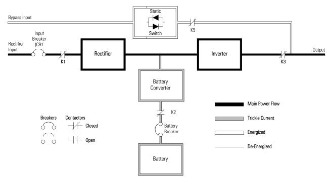
Figure 6-2. Path of Current Through the UPS in Online Mode
