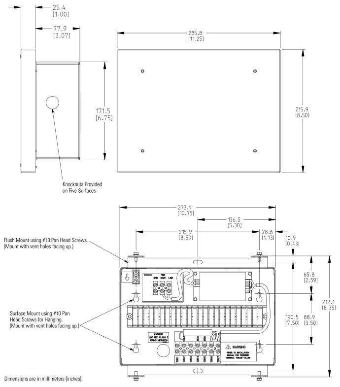
Figure 5-14. Supervisory Contact Module II Dimensions
