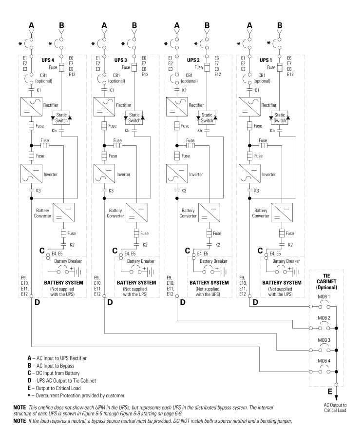
Figure 6-15. Typical Distributed Bypass System (3+1 and 4+0 Configurations)
