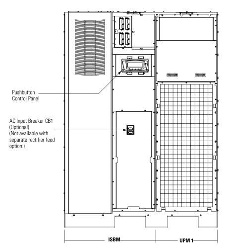
Figure 7-1. UPS Controls and Indicators
