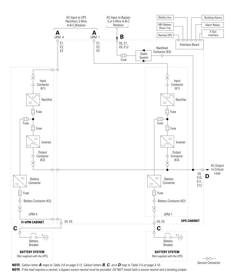
Figure 6-8. UPS System with Field Installed UPM – Separate Rectifier Feed, Separate Battery, Dual-Feed Configuration
