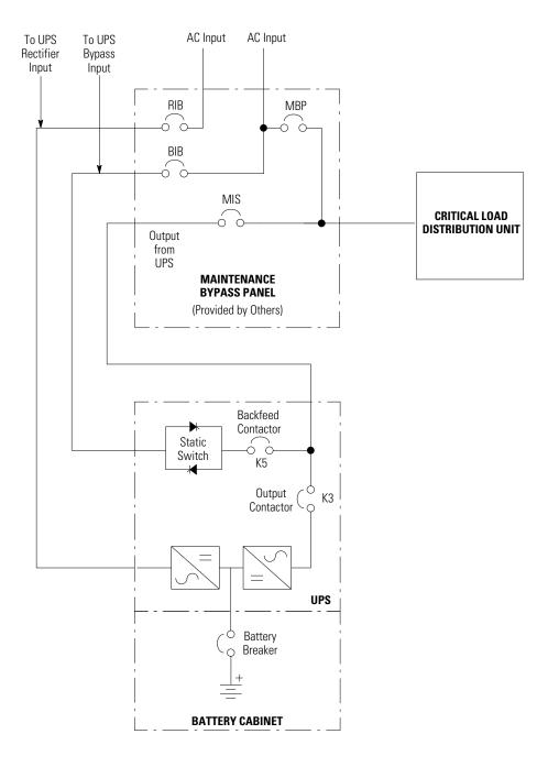
RIB: Rectifier Input Breaker
