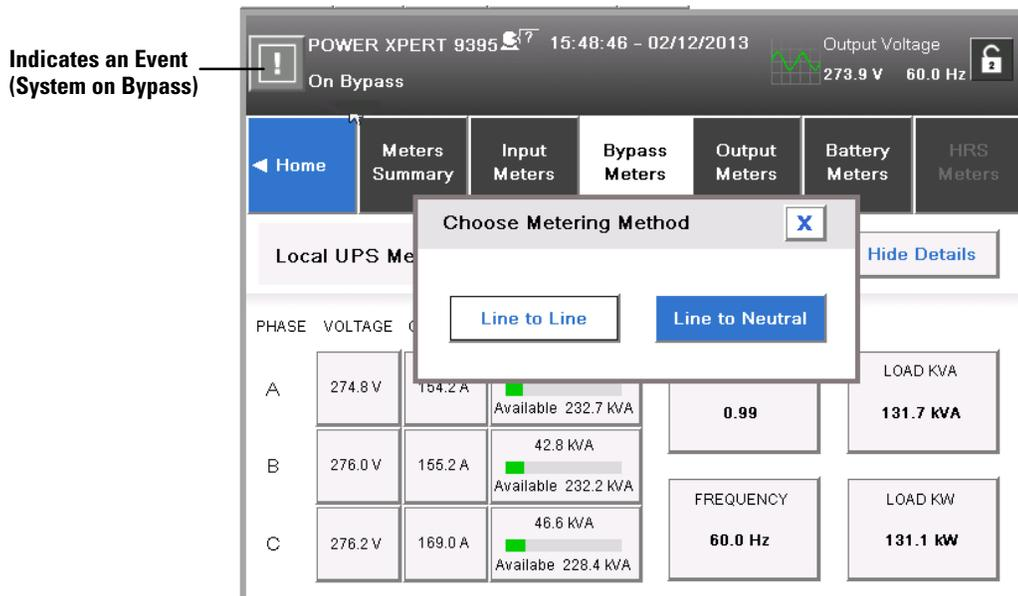
Figure 7-37. Bypass Mode Metering Method Option Screen
