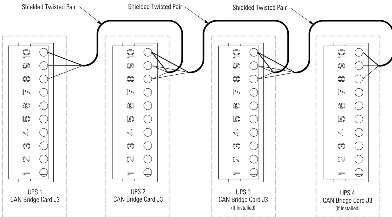
**NOTE** External CAN connections between UPSs require shielded twisted-pair wire.
