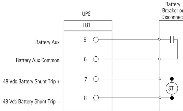
**NOTE** Battery Aux and DC Shunt Trip wiring should be a minimum of 18 AWG.
