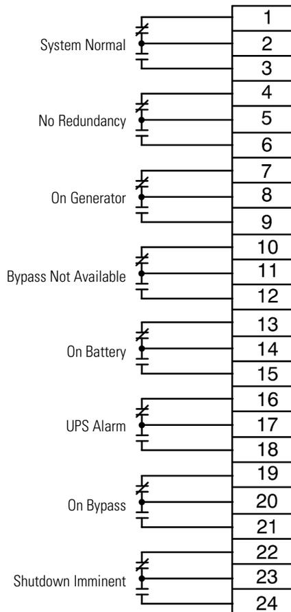
**Figure 5-11. Supervisory Contact Module II TB2**
