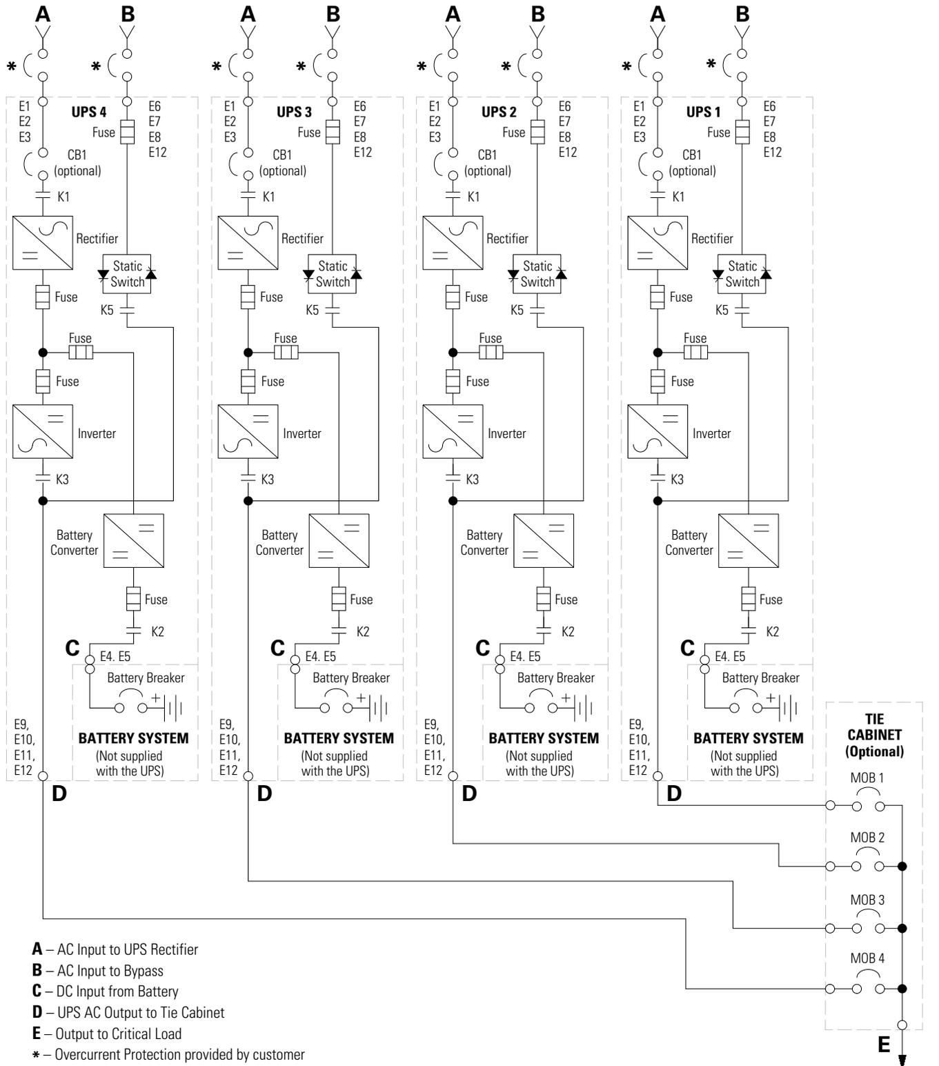
**NOTE** This oneline does not show each UPM in the UPSs, but represents each UPS in the distributed bypass system. The internal structure of each UPS is shown in Figure 6-5 through Figure 6-8 starting on page 6-8.
