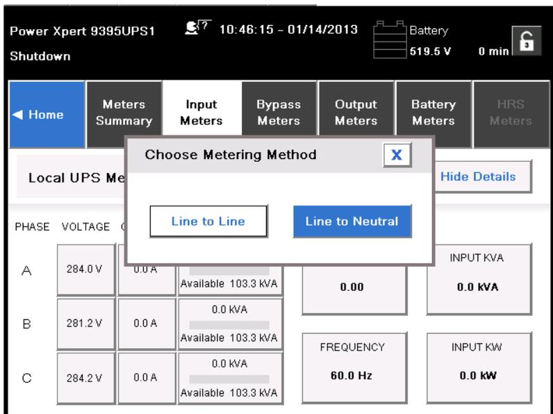
Figure 7-36. Online Mode Metering Method Option Screen
