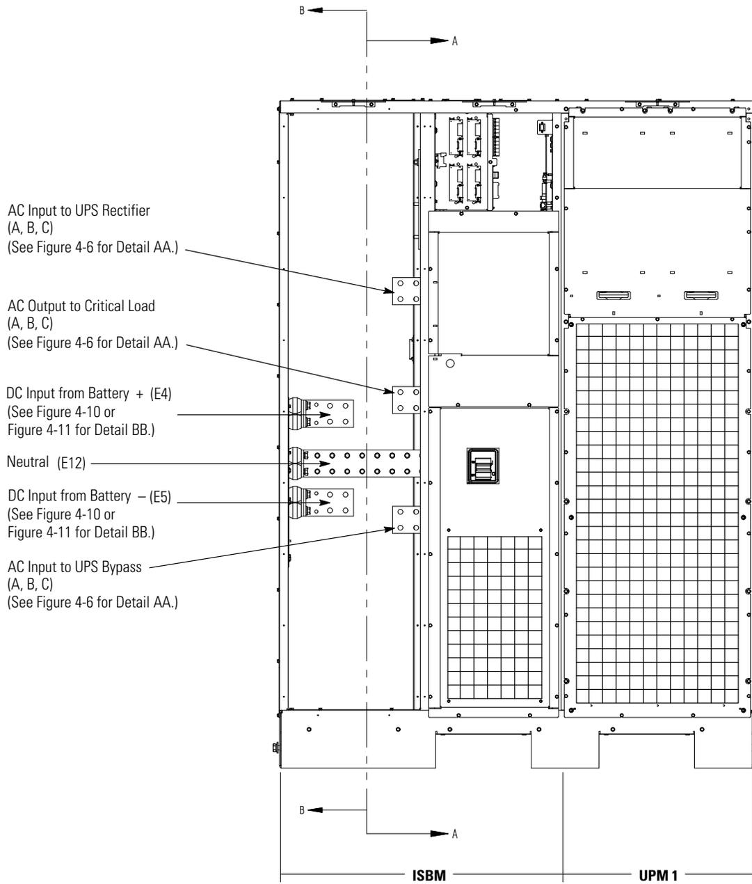
Figure 4-5. UPS Power Terminal Locations – Common Rectifier Feed
