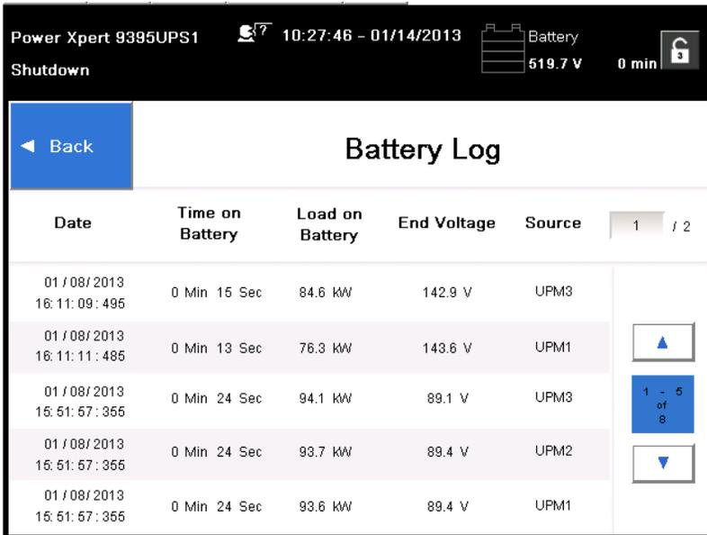
Figure 7-28. Battery Log Detail
