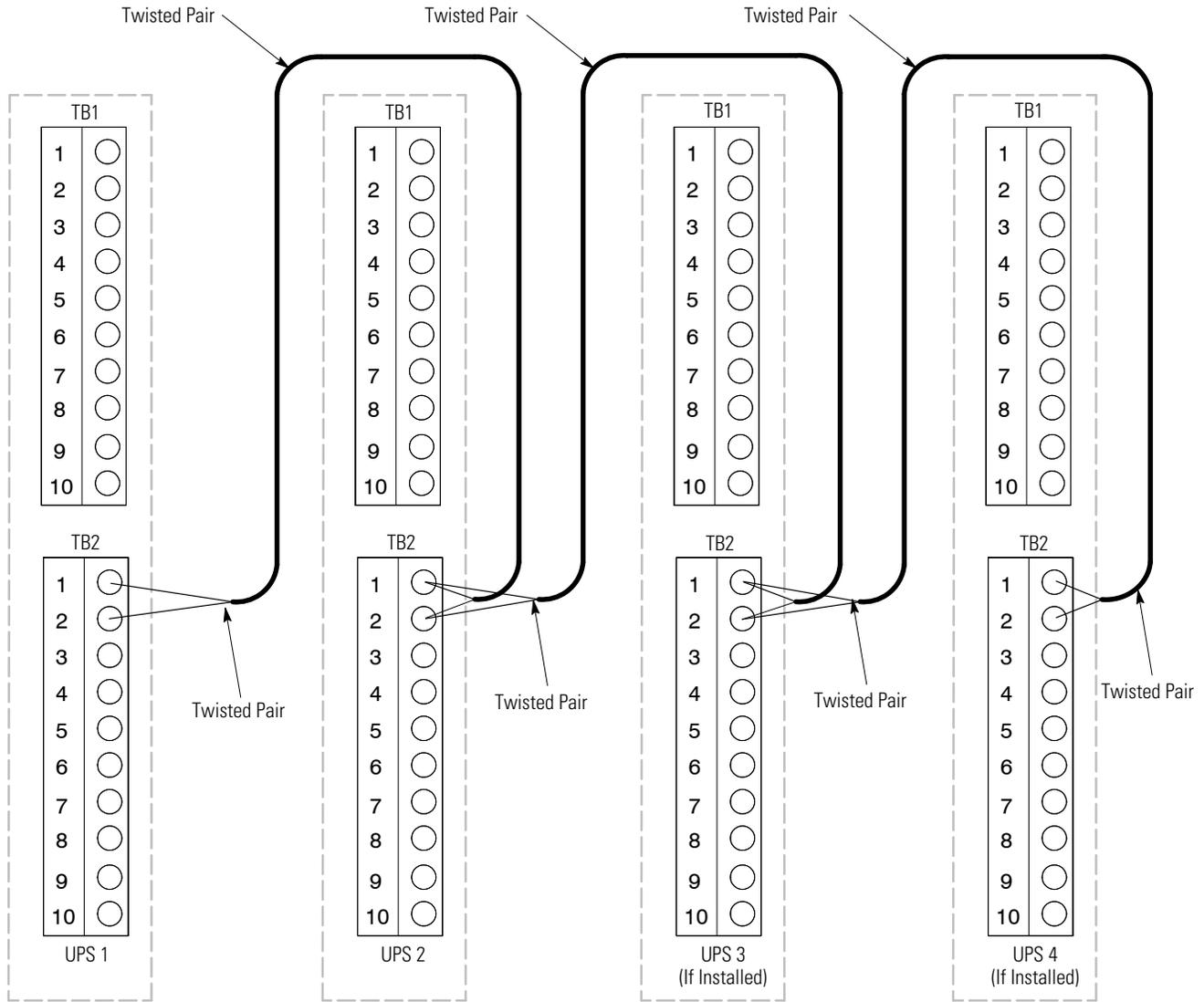
**NOTE** Use twisted-pair wiring between the UPS and MOB AUX contacts.
