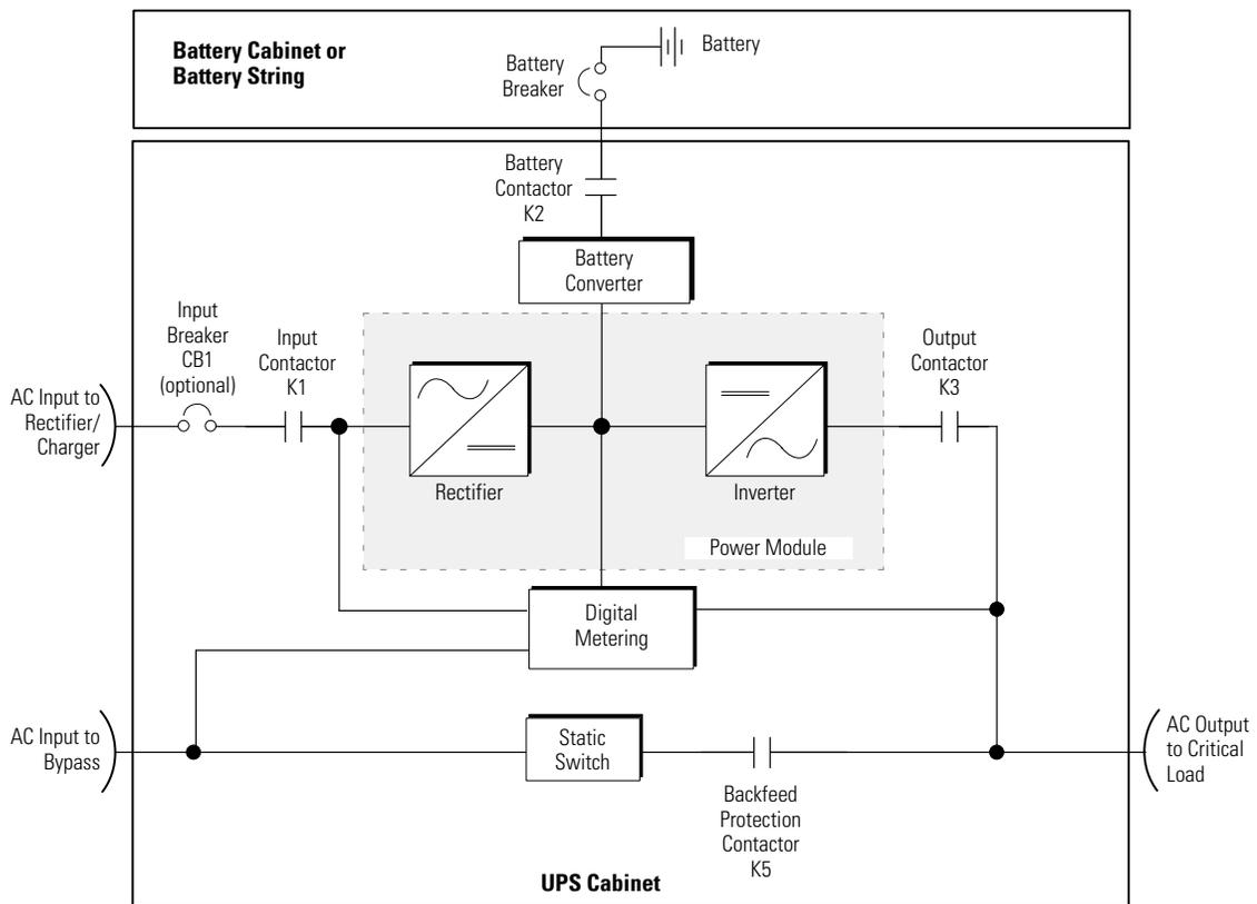
Figure 6-1. Main Elements of the UPS System
