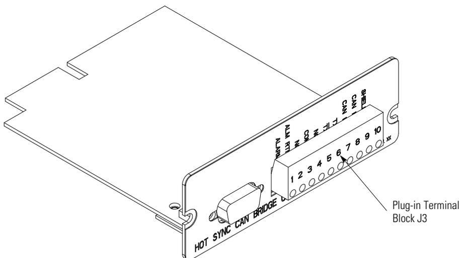
**Figure 5-1. Powerware Hot Sync CAN Bridge Card**
