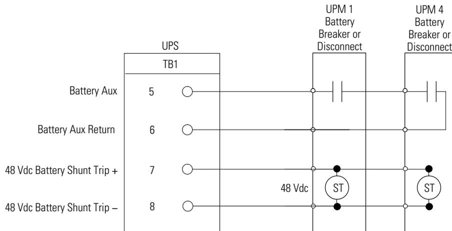
**NOTE** Battery aux and DC shunt trip wiring should be a minimum of 18 AWG.
