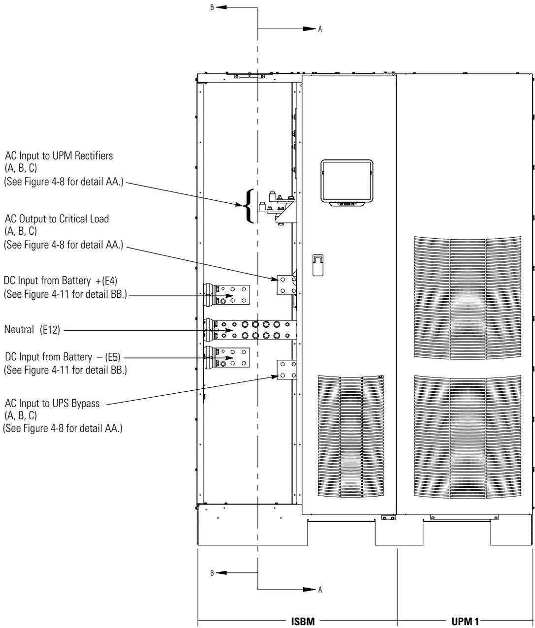
Figure 4-7. UPS Power Terminal Locations – Separate Rectifier Feed
