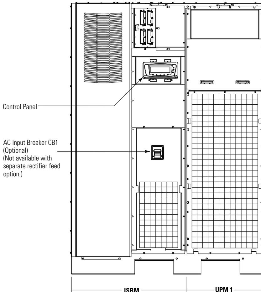
Figure 7-1. UPS Controls and Indicators
