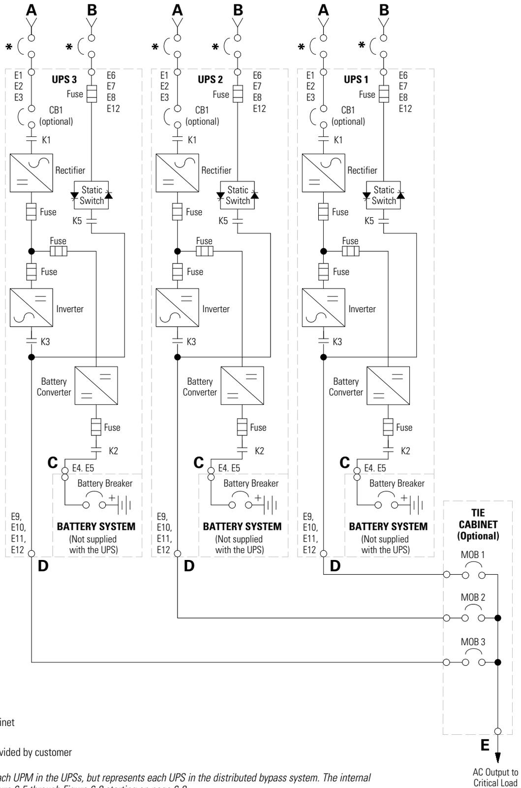
**Figure 6-14. Typical Distributed Bypass System (2+1 and 3+0 Configurations)**
