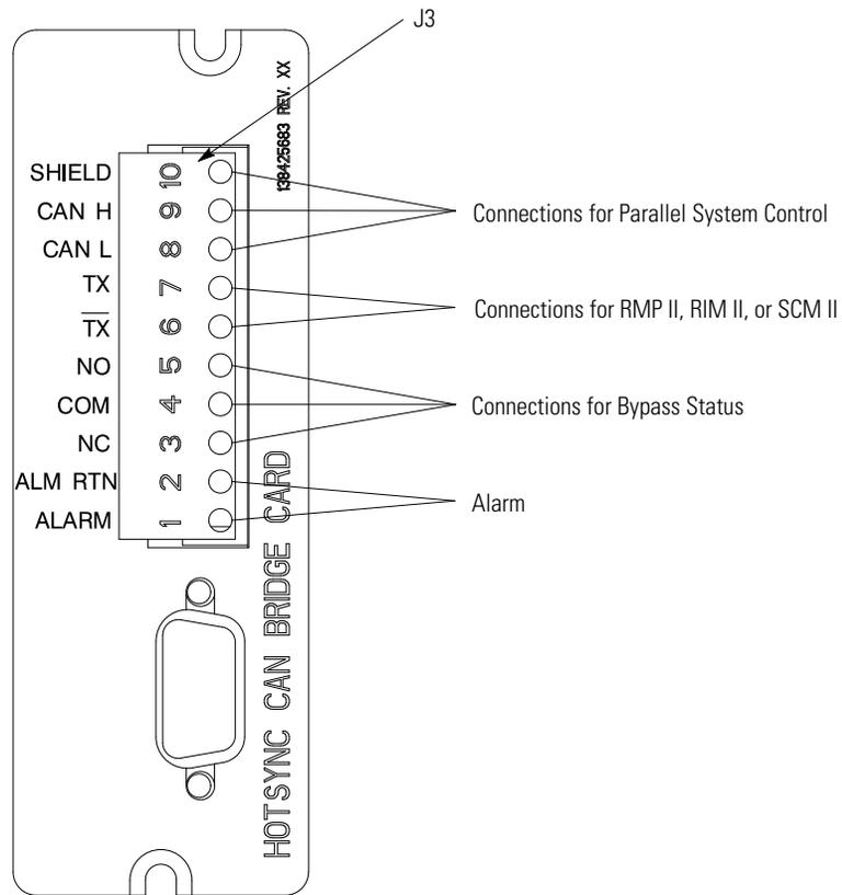
Figure 5-2. Powerware Hot Sync CAN Bridge Card Connections
