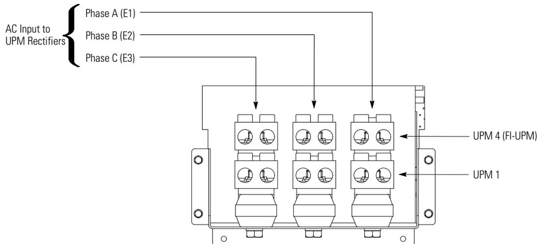
Figure 4-9. UPM Rectifier Input Power Terminal Block Detail
