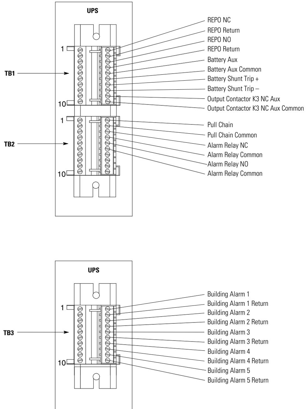
**NOTE** All building alarm inputs require an isolated normally-open or normally-closed contact or switch (rated at 24 Vdc, 20 mA minimum) connected between the alarm input and common terminal as shown. Building alarm inputs can be programmed for use with either normally-open or normally-closed contacts. All control wiring and relay and switch contacts are customer-supplied.
