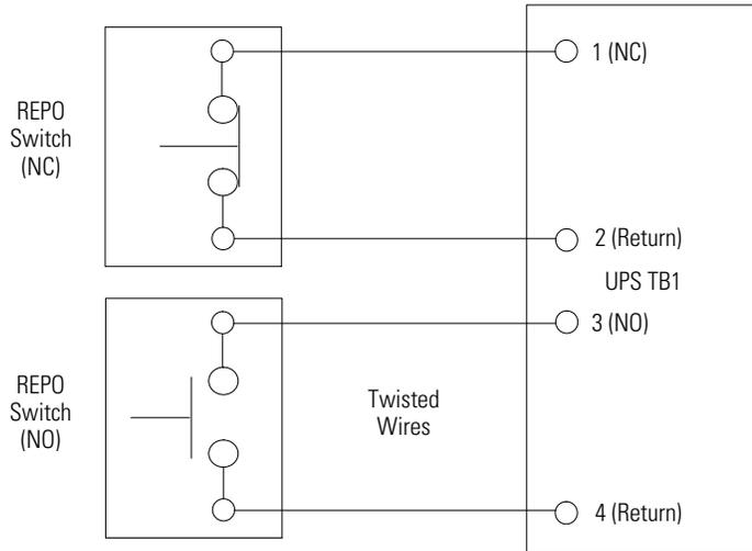
**NOTE** REPO switch rating is 24 Vdc, 1A minimum.
