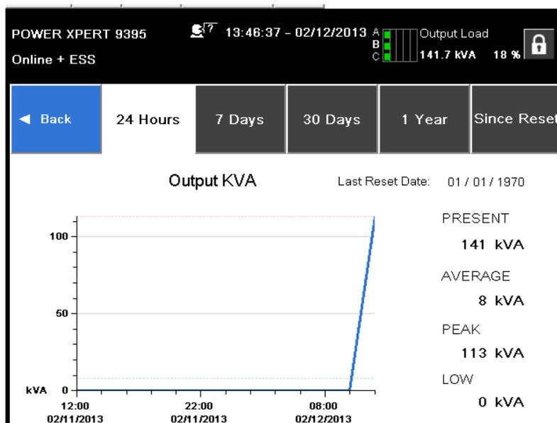
Figure 7-15. Output kVA Screen from Home Screen
