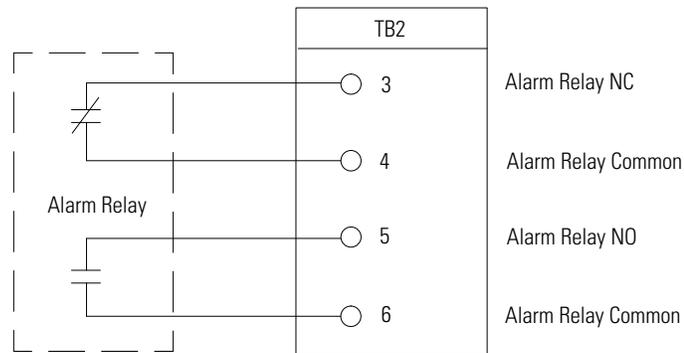
**NOTE** Alarm relay contacts have a maximum current rating of 5A and a switched voltage rating of 30 Vac and 28 Vdc.
