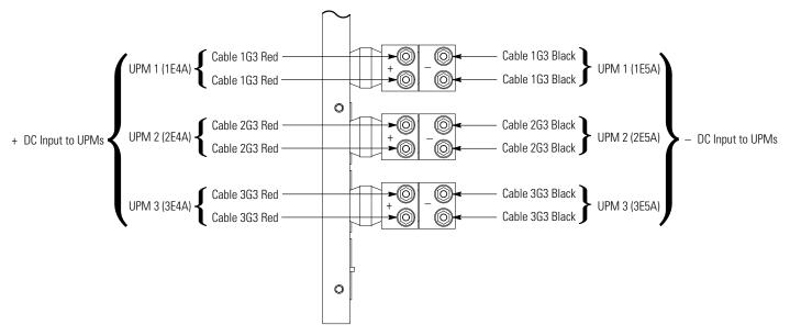
Figure 4-10. ISBM Section Battery Input Power Terminal Detail
