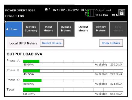
Figure 7-23. Output Meters Screen
