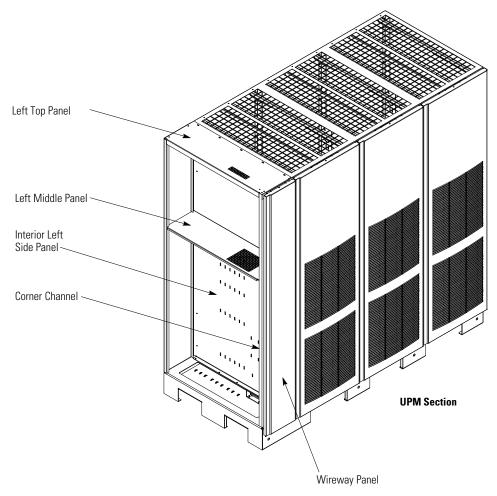
Figure 4-5. Section Joining
