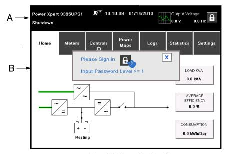
Figure 7-11. Parts of the Touch Screen
