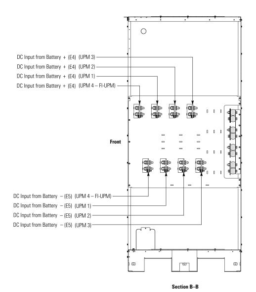
Figure 4-20. ISBM Section Power Terminal Detail BB – Separate Battery
