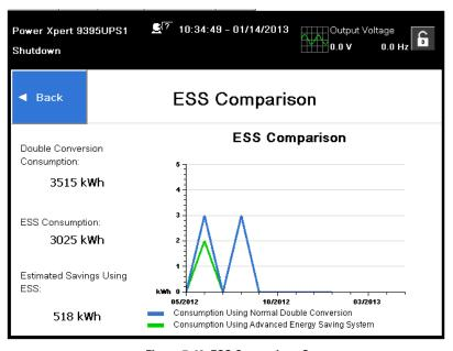
Figure 7-46. ESS Comparison Screen
