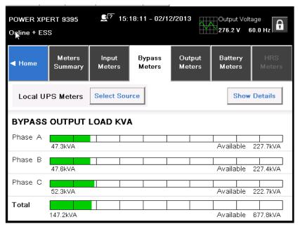
Figure 7-22. Bypass Meters Screen
