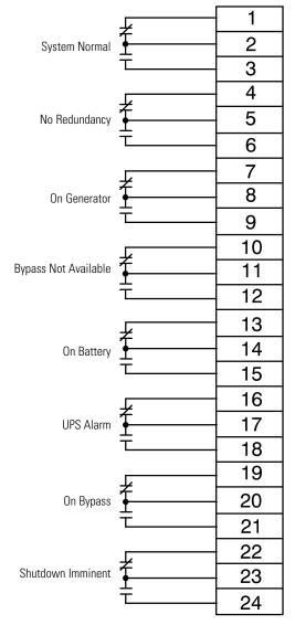
Figure 5-11. Supervisory Contact Module II TB2
