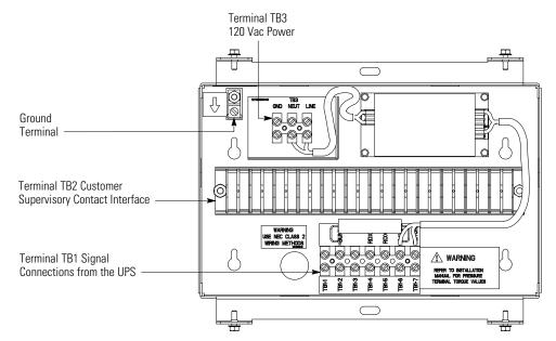
Figure 5-10. Supervisory Contact Module II Terminal Location
