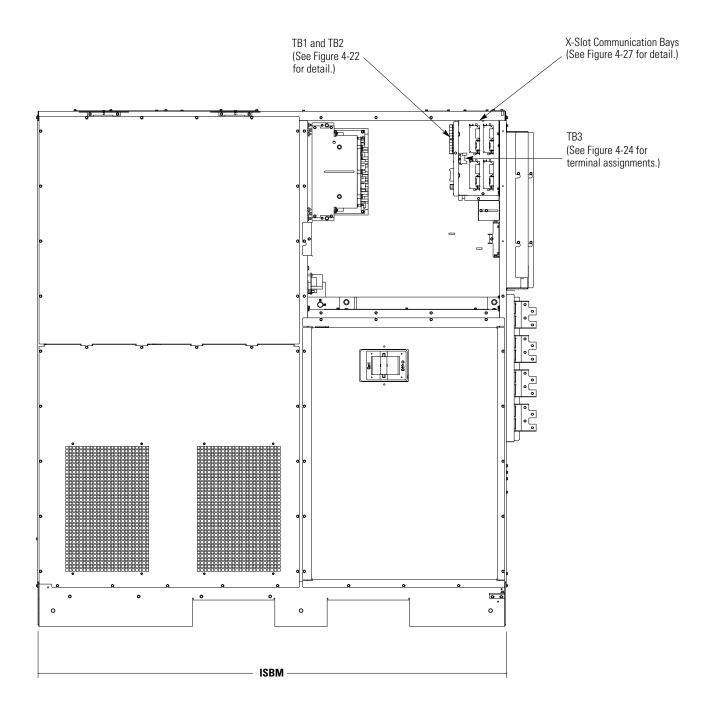
Figure 4-21. ISBM Section Interface Terminal Locations
