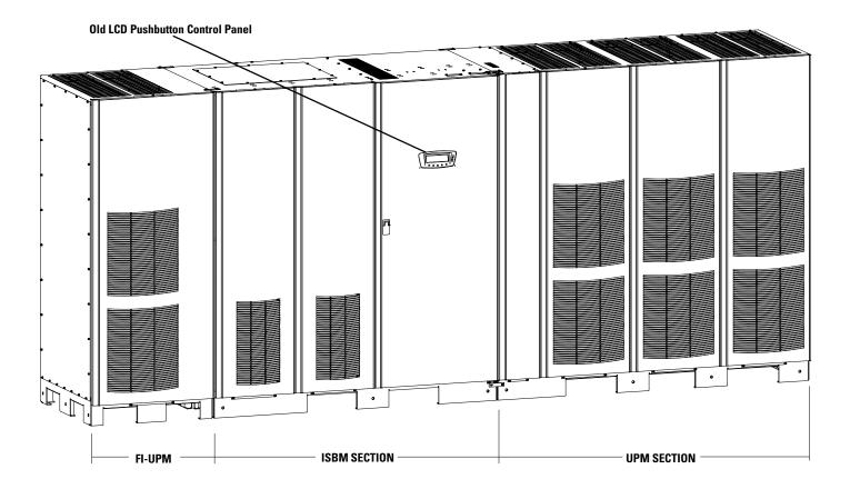
Figure 1-1. Power Xpert 9395 Four UPM UPS (1000–1100 kVA)
