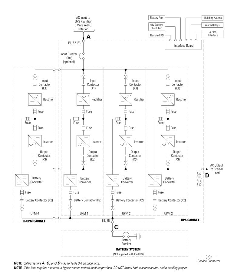
Figure 6-9. UPS System – Four UPM Common Rectifier Feed, Common Battery, IOM Configuration
