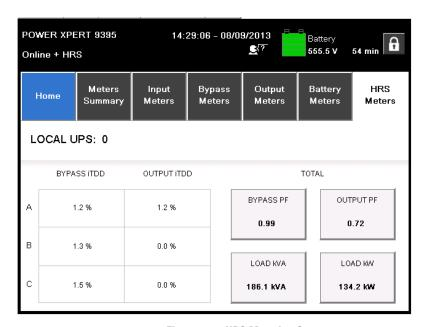
Figure 7-42. HRS Metering Screen
