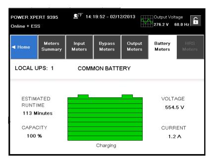
Figure 7-26. Battery Meters Screen
