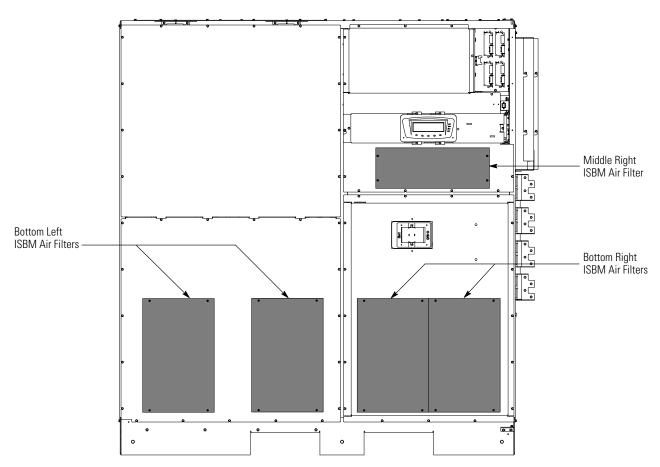
Figure 9-1. ISBM Section Air Filter Locations – Continuous Static Switch
