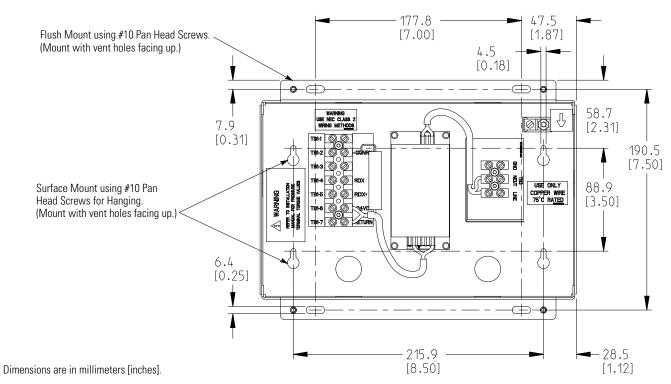
Figure 5-12. Remote Monitor Panel II Dimensions
