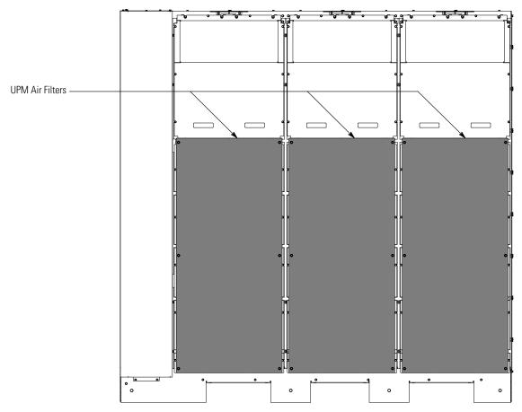
Figure 9-2. UPM Section Air Filter Locations
