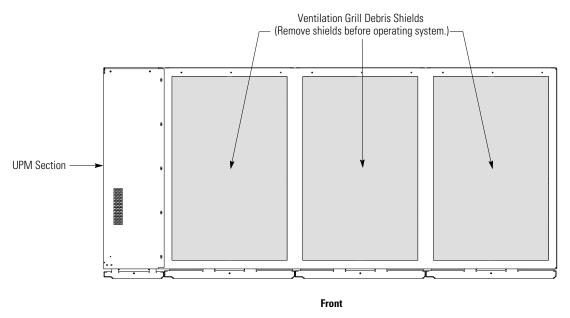
Figure 4-15. ISBM and UPM Section Debris Shields
