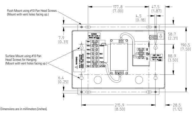
Figure 5-13. Relay Interface Module II Dimensions
