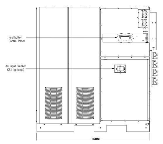
Figure 7-1. UPS Controls and Indicators
