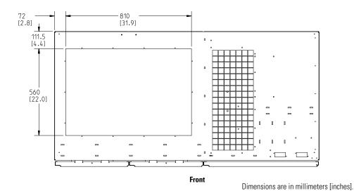
Figure 3-7. ISBM Section Dimensions (Top View)
