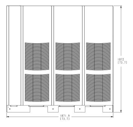
Figure 3-5. UPM Section Dimensions (Front View)
