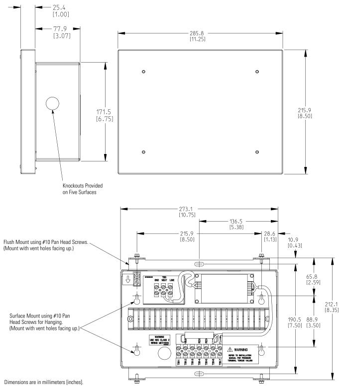
Figure 5-14. Supervisory Contact Module II Dimensions
