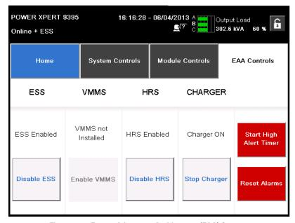
Figure 7-40. Energy Advantage Architecture (EAA) Screen
