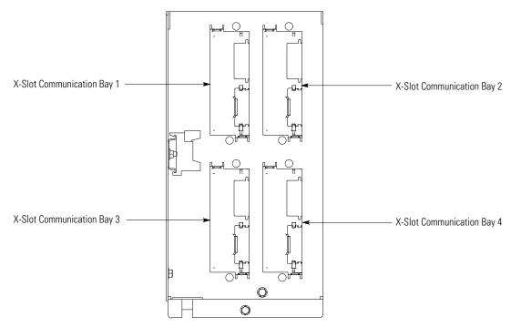
Figure 4-27. X-Slot Communication Bays
