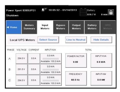
Figure 7-24. Input Meters Detail Screen
