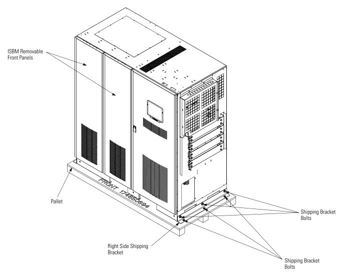
Figure 4-2. Removing the ISBM Section Right Side Shipping Bracket
