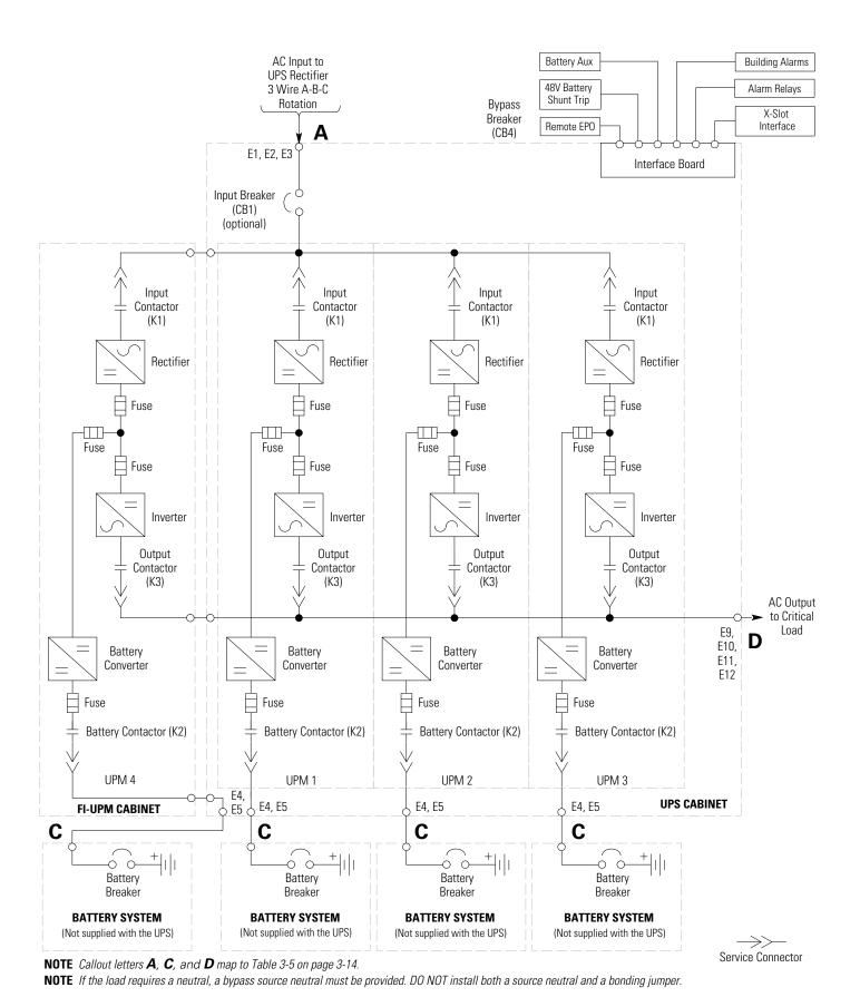
Figure 6-10. UPS System – Four UPM Common Rectifier Feed, Separate Battery, IOM Configuration
