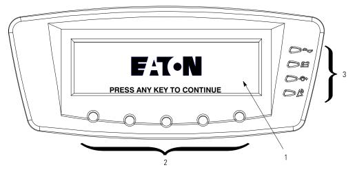
Figure 7-2. UPS Control Panel
