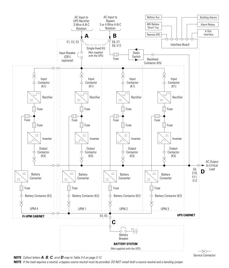
Figure 6-5. UPS System – Four UPM, Common Rectifier Feed, Common Battery, Dual-Feed Configuration, Continuous Static Switch
