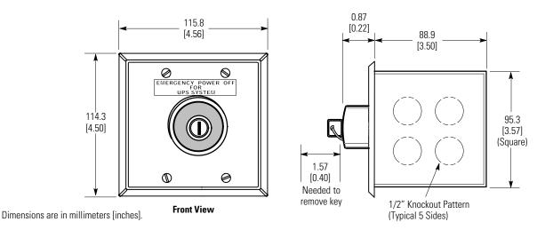
Figure 3-11. Remote EPO Switch Dimensions
