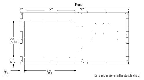
Figure 3-8. ISBM Section Dimensions (Bottom View)
