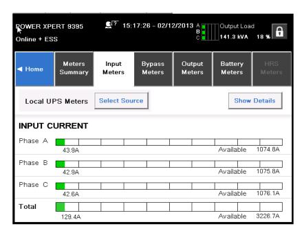
Figure 7-21. Input Meters Screen
