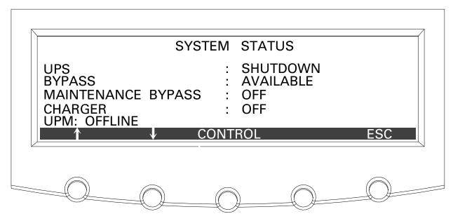
Figure 7-6. Typical System Status Screen
