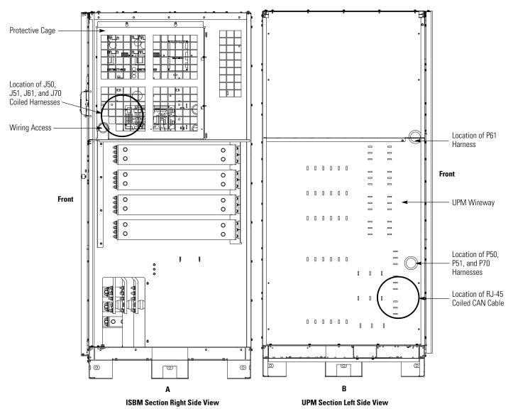
Figure 4-12. UPS Intercabinet Interface Harness Locations
