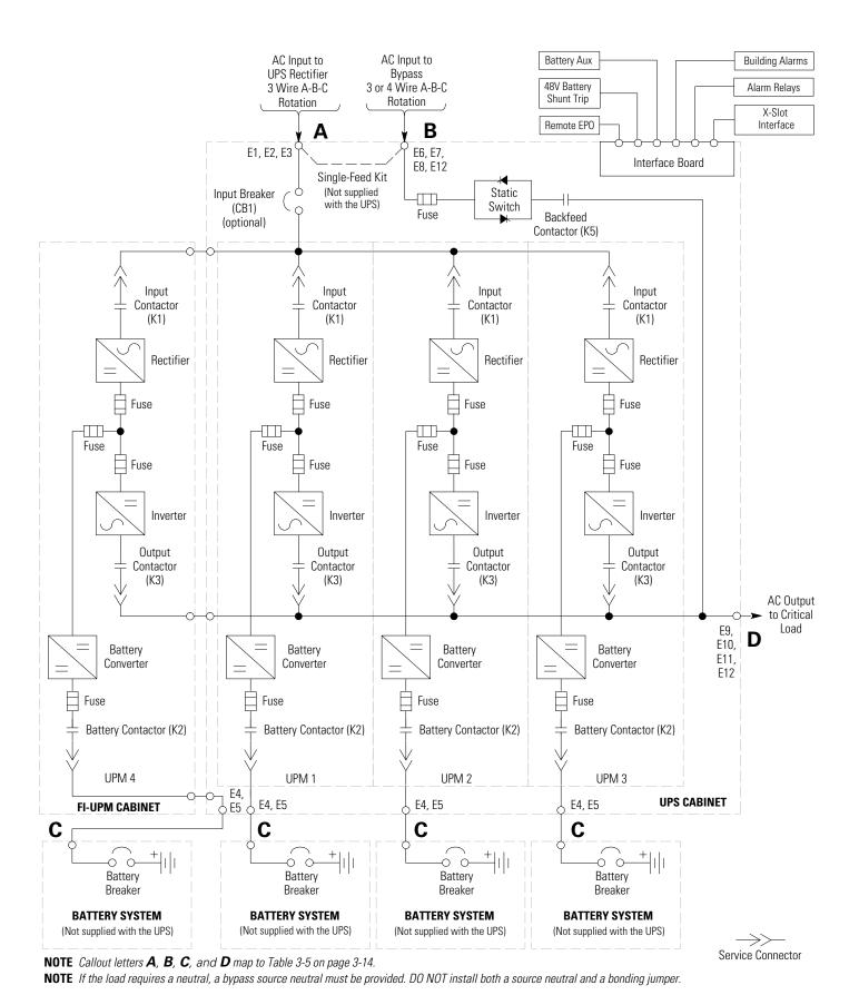
Figure 6-6. UPS System - Four UPM, Common Rectifier Feed, Separate Battery, Dual-Feed Configuration, Continuous Static Switch
