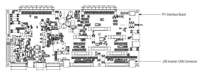
Figure 4-14. J39 Location on PI1 Interface Board
