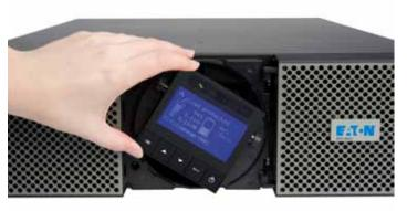
The 9PX displays key data such as its ≥93 percent efficiency rating, alarm history, runtime remaining, load percentage and more in a graphical format.
