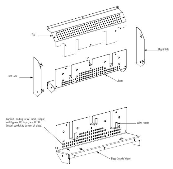
Figure 4-5. UPS Power Terminal Cover Parts
