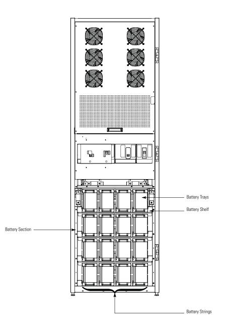
**NOTE** The Eaton 9E-40 model has battery strings installed on three shelves. The Eaton 9E-60/40 and Eaton 9E-60/60 models have battery strings installed on four shelves.
