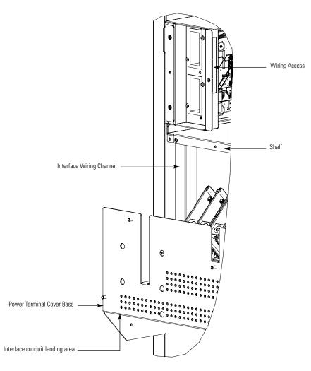
Figure 4-14. Interface Conduit Landing and Wiring Channel
