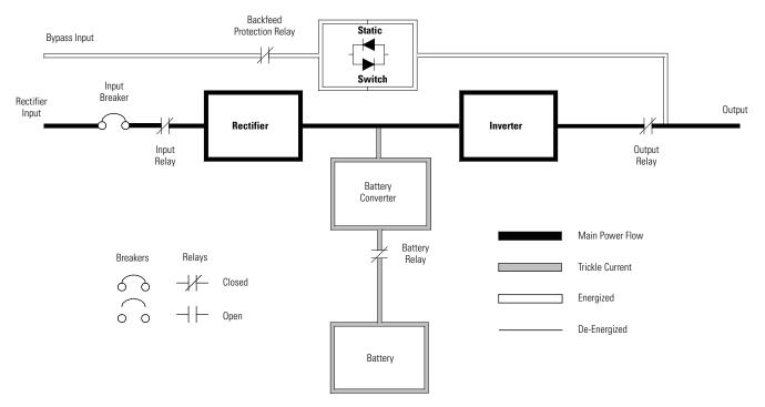
If the utility AC power is interrupted or is out of specification, the UPS automatically switches to Battery mode to support the critical load without interruption. When utility power returns, the UPS returns to Normal mode.
