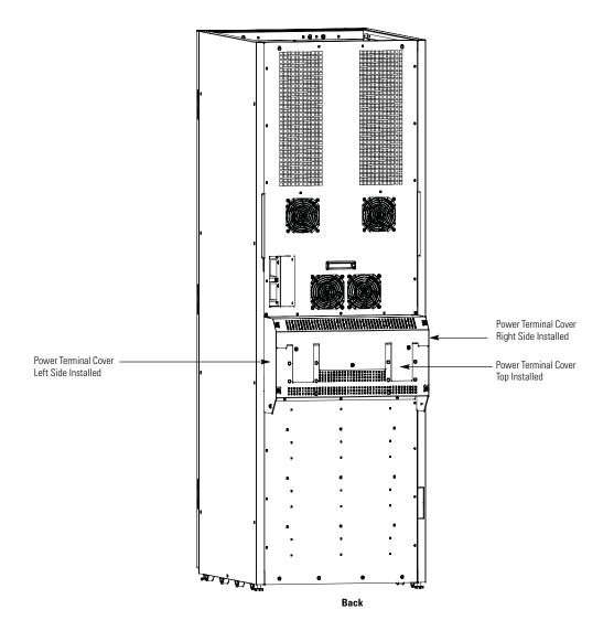
Figure 4-9. Power Terminal Cover Top Installation
