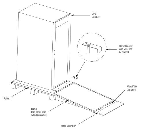
Figure 4-2. Attaching the Ramp to the Pallet
