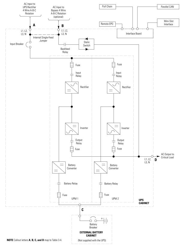
Figure 5-6. UPS System Oneline – External Battery
