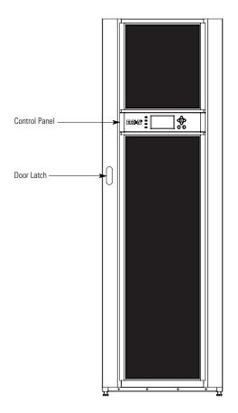
Figure 6-1. UPS Controls and Indicators
