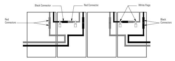
Figure 4-24. Battery String Connections
