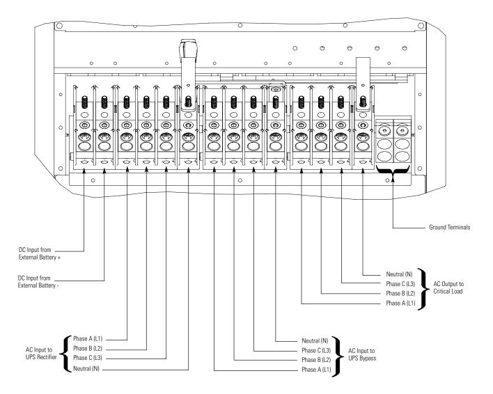
Figure 4-8. Power Terminal Detail
