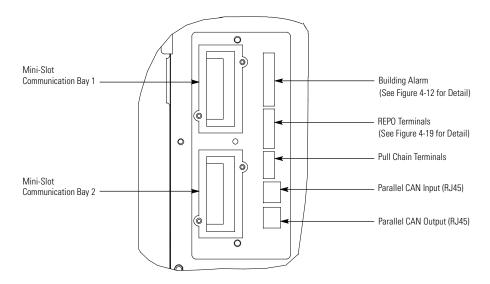
Figure 4-11. Interface Terminal Detail (Terminal Cover Removed)
