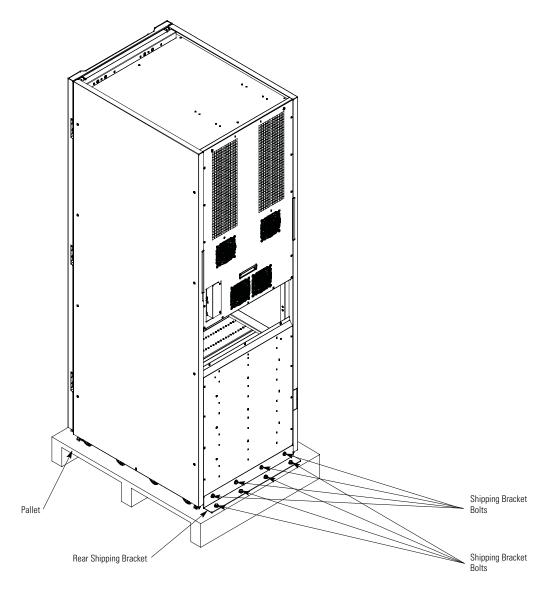
Figure 4-3. Removing the Rear Shipping Bracket
