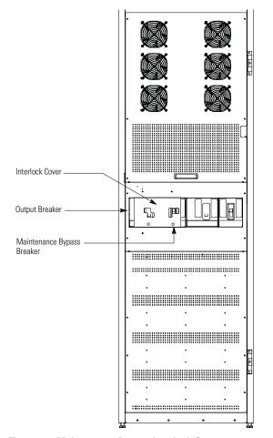
Figure 6-8. Maintenance Bypass Interlock Cover
