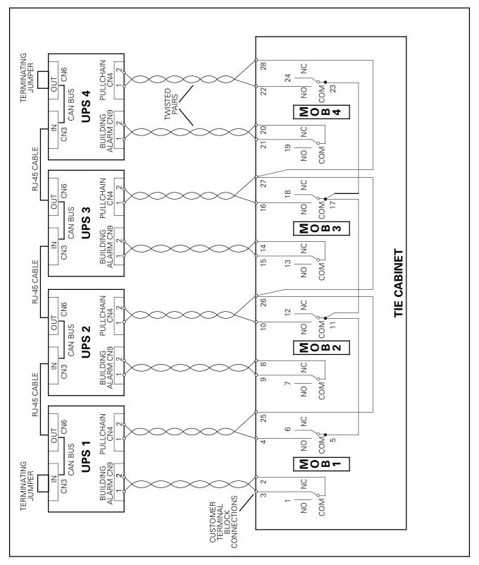
Figure 4-17. Parallel UPS Control Wiring
