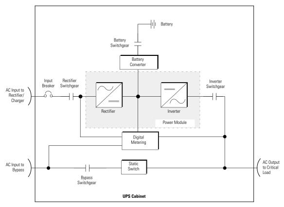
Figure 5-1. Main Elements of the UPS System
