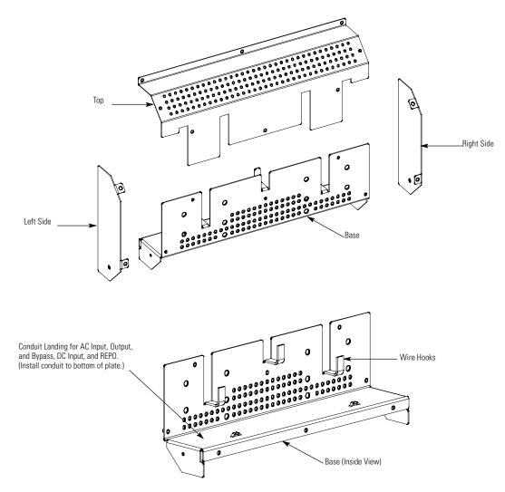
Figure 4-5. UPS Power Terminal Cover Parts
