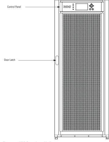
Figure 6-1. UPS Controls and Indicators
