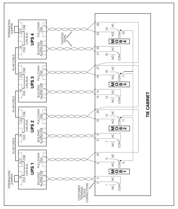
Figure 4-17. Parallel UPS Control Wiring
