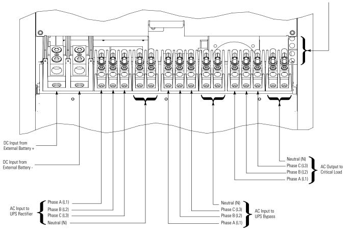
Figure 4-8. Power Terminal Detail
