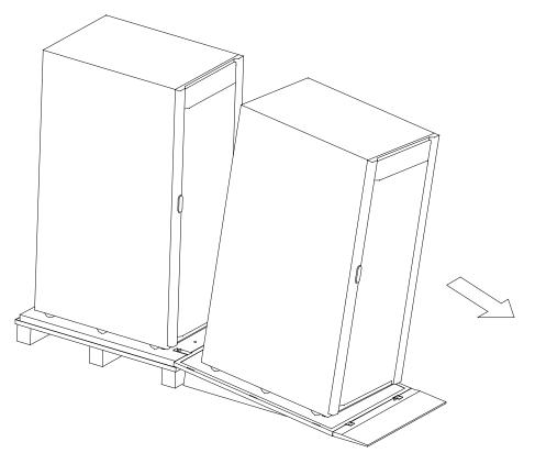
Figure 4-4. Rolling the Cabinet Down the Ramp
