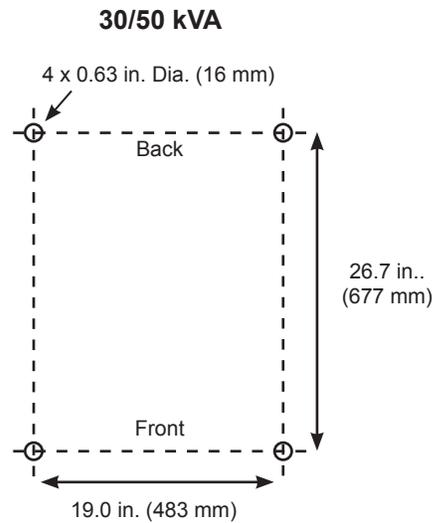
**FIGURE 8.3 HOLE LOCATIONS/DIMENSIONS ON BOTTOM OF UPS**
