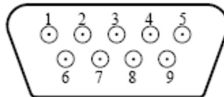
**NOTE:** Pin switches are shown in their inactive states. For example, if battery voltage is low, pin 7 will be connected to pin 5. Pin number 3 is not used.
